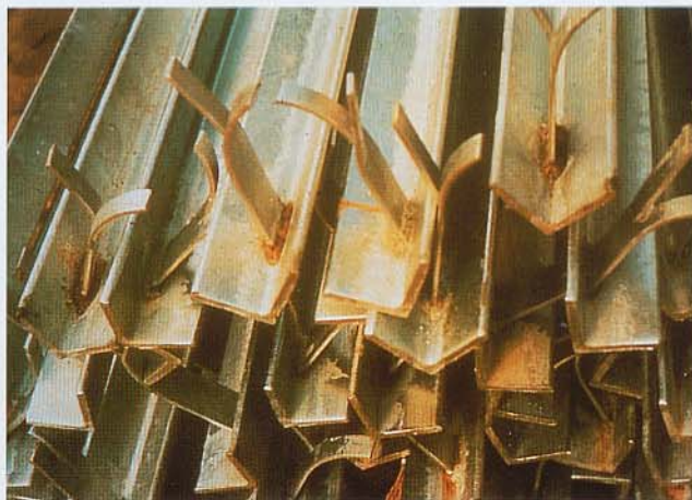
Fig. 2: Defects in galvanized coating due to presence of welding slag.
