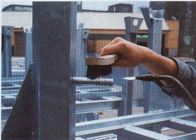
Fig. 3: Threads can be cleaned by reheating so that the zinc melts followed by brushing.
