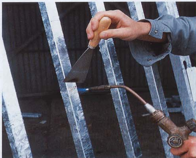
Fig. 1: Zinc runs can be removed by reheating the area and then brushing off superfluous zinc or removing it with a spatula.
